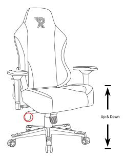
EN: Seat height adjustment (Adjusting knob on the right)
