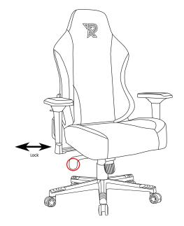
**EN:** Rocking: Pull out the handle to start rocking. Insert to stop rocking
